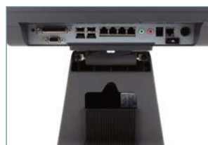
Stand with adapter housing and cable management
