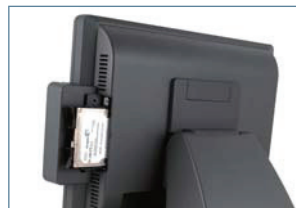
Slide in/out HDD replacement
